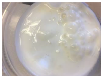
Figure 5. Totally non-acceptable foams that must be discarded. New dispersion must be used to prepare a new foam.
