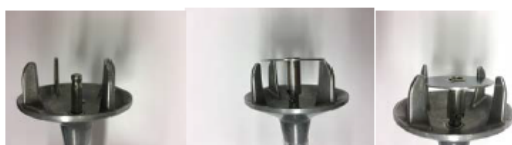
Figure 1. Head of the blender with spike where the blade is connected by pressing. Head of blender with no blade (left), head of the blender with the blade on but NOT correctly put (middle), head of the blender with the blade correctly put since the spike is completely at the end of the hole in the blade (right).
