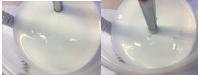
Figure 8. Very good foams with no small visible bubbles (left), or only few big bubbles (right) that can be very easily removed with a Pasteur pipette.
