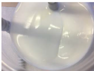
Figure 7. Acceptable foam with only few (from 1 to 5) small visible bubbles.
