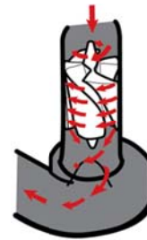
Figure 4: Secondary flow path
