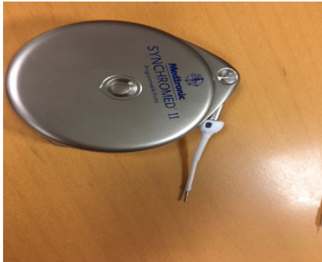
Figure 3: Medtronic connector catheter is cut and a metal phalange is inserted into the connector to allow for connection to the Codman Catheter.
