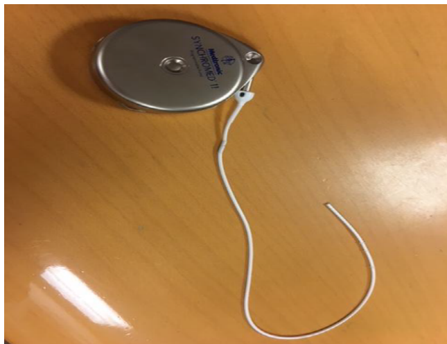
Figure 4: The Codman catheter is now connected to the Medtronic pump using the metal phalange.
