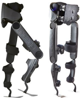
(Figure 1) Indego® ; total weight 26 pounds, 5 modular components, powered assist at the hip and knee joints, carbon fiber ankle foot orthoses is passive.
