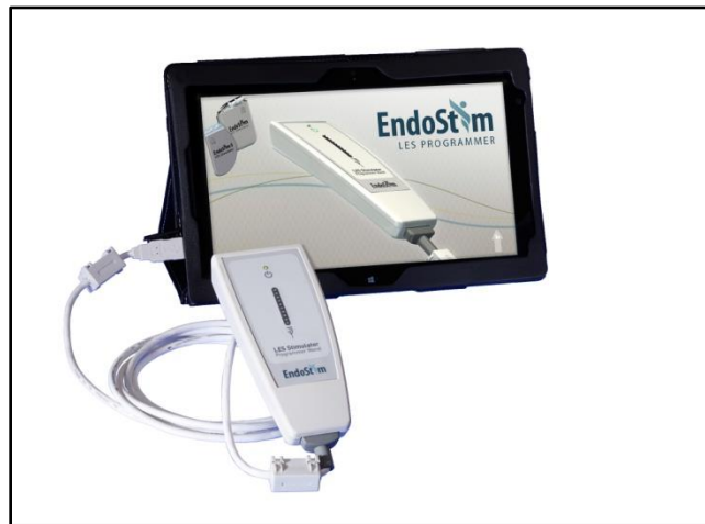
Figure 3. Tablet PC with EndoStim Programmer Software and USB Programmer Wand
