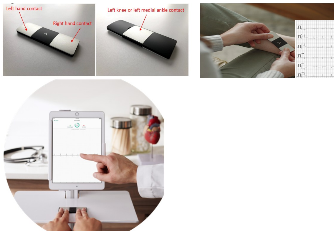
Figure 3. AliveCor 6L wireless ECG device with portable 6-lead ECG displayed
