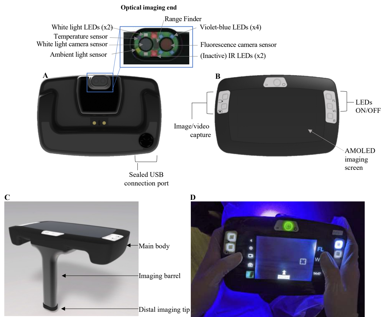
Figure 10.1 Handheld Fluorescence Camera Renderings of the (A) front (target-facing), (B) back (user-facing) and (C) side of the Handheld Fluorescence Camera, including the distal imaging tip (A, inset) and the mechanical buttons which control image/video capture, imaging mode, and device power (B). (D) Representative photograph of user-facing side of Handheld Fluorescence Camera being used to perform fluorescence imaging in a dark environment.
