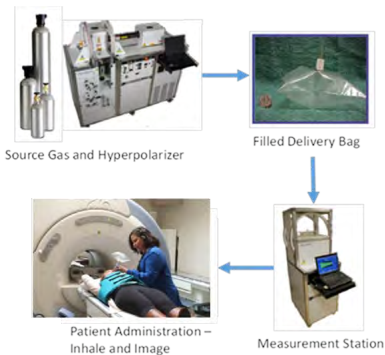
Figure 2 Depiction of the Hyperpolarization Process and Device Components
